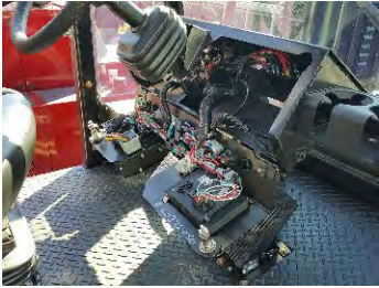
Flip-down Dash with Color/Number Coded Wiring (Standard)
