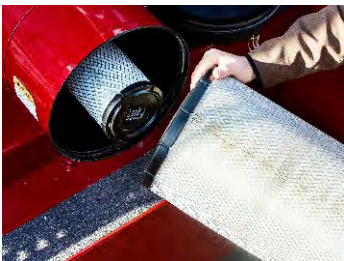
Donaldson Air Cleaner with Safety Element (Standard)
