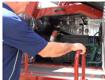
Service & Inspections from Running Board Dual Engine Bay Doors provide full access
